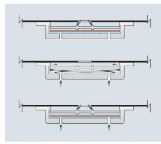
The sealant and the membrane prevent air from entering the packaging.
